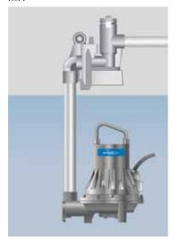
Stationary wet installation with the pump suspended from the discharge pipe. The quick connection joint has an integrated non-return valve.
