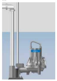
Stationary wet installation with guide bars and automatic discharge connection bolted to the sump floor. When lowering a pump with guide bars, the pump automatically locks to, and is released from, the discharge connection. МН
